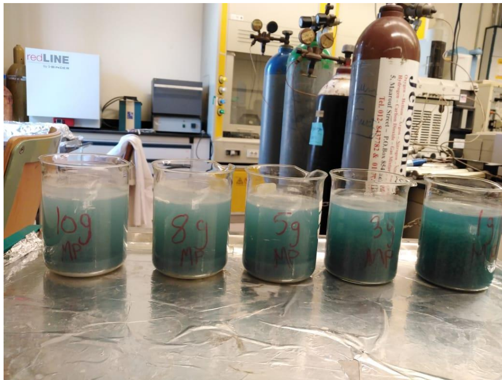
Figure 4.6: Effect of MP dosages on the Color of the Solution
