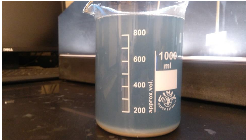
Figure 4.5: Effect of 1g CKD on the Color of the Solution
