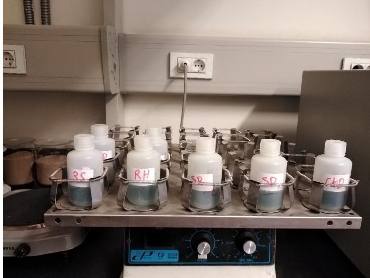
Figure 3.2: HDP Bottles on the mechanical orbital
